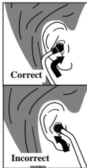
Your new Littmann stethoscope is designed to provide a comfortable acoustically sealed ear fit. Notice that the ear-tubes are set to accommodate the typical anatomy of the ear canal. The eartips should point in a forward direction as you insert them into your ear canals.
