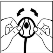
With the diaphragm side up, push the rim at the apex with both thumbs and roll the rim off the edge of the chestpiece. Remove the diaphragm from the rim and clean parts in soapy water or
