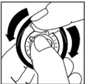
Using your fingertip, apply a small amount of talcum powder to the inside surface of the flexible edge of the diaphragm then align the rim and diaphragm as a unit. This will facilitate assembly and maintain smooth and quiet low/high frequency alternation. Snap the diaphragm with your fingers to remove excess talcum powder. Insert the flexible edge of the diaphragm into the groove of the rim. This is best accomplished by starting with the rim positioned above the legible side of the
